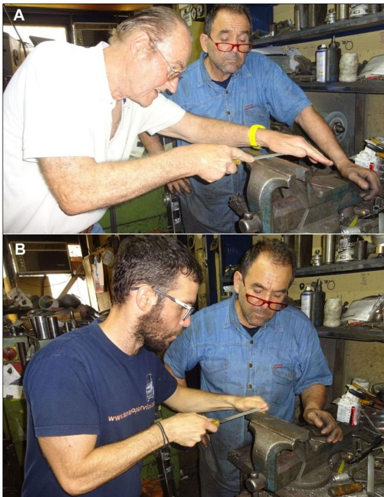
Figure 11. A) The author during filing. He is able to file a plane. B) Sotiris is not able to file a plane. As the teacher/father said, also his posture during filing is wrong.
